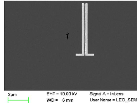
Figure 1: SEM image of folded CPS structure
