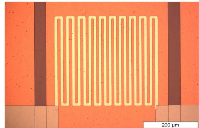
Optical microscope image of fabricated RTD
