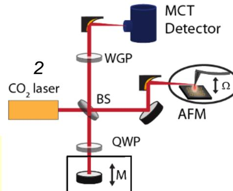
Figure 2: Schematic of the SNOM setup
