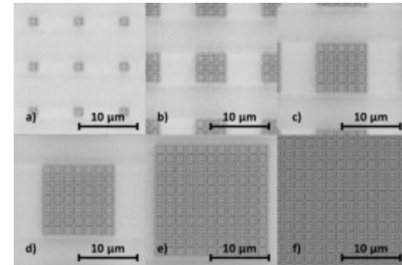
SEM micrograph of truncated arrays as well as a quasi-infinite array.
