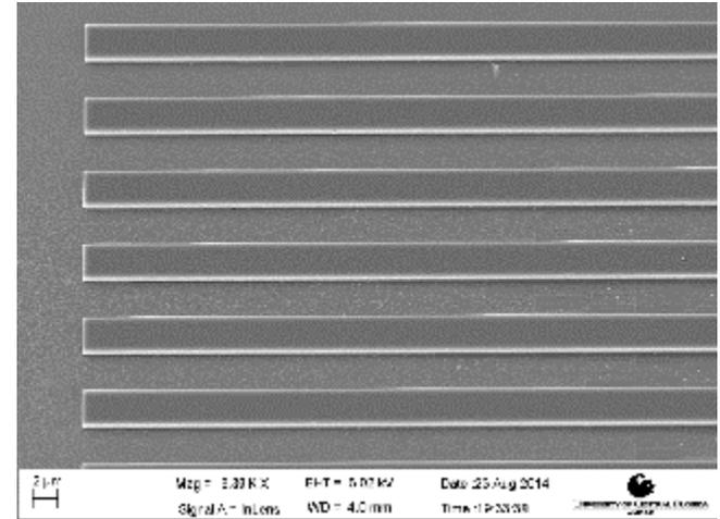
Figure 1. Array of PMMA channel waveguides.
