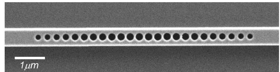
*Top: photonic crystal micro-ring resonator for low-energy optical modulation and bio-sensing applications.*
