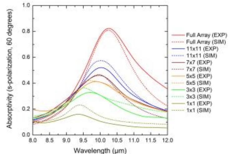
Spectral absorptivity of the truncated arrays as well as the full (quasi-infinite) array.
