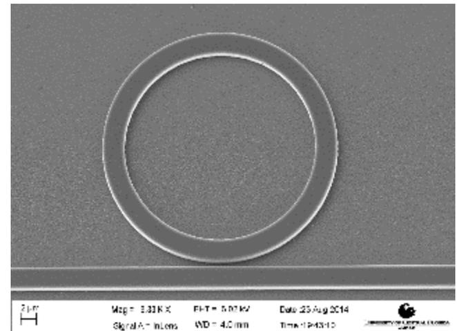
Figure 2. PMMA ring resonator and channel waveguide
