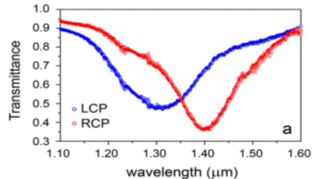
Plot of left circular polarized and right circular polarized light normally incident on the metamaterial structure. The structure demonstrates large circular dichroism.
