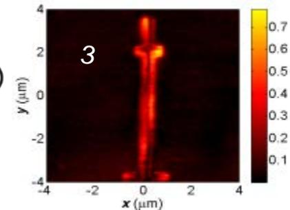
Figure 3: Instantaneous field measurement of Folded CPS structure with s-SNOM;
