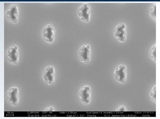
tool = STS SOE recipe = DKB\_INSB Ar = 5 sccm CH4 = 15 sccm H2 = 50 sccm ICP = 600 W RIE = 150 W press = 7 mTorr
