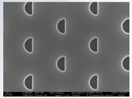
tool = Plasma Therm ICP, left chamber recipe = DKB\_SI 16 sccm Cl2 4 sccm Ar press = 5 mTorr 50 W RIE 200 W coil
