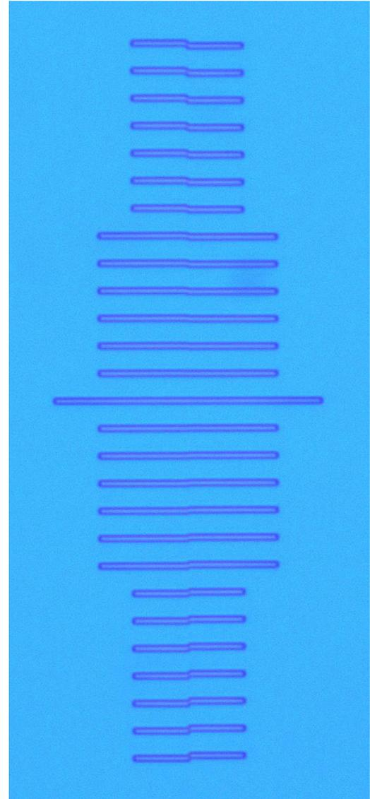
After examining the field boundary of the Vernier pattern, there appears to be less than 20nm of stitching error well within spec.
